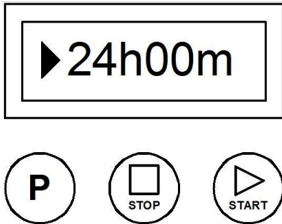
Fig 2. Depending on previous settings, the display will show the previously set operating time for the creaming machine.
